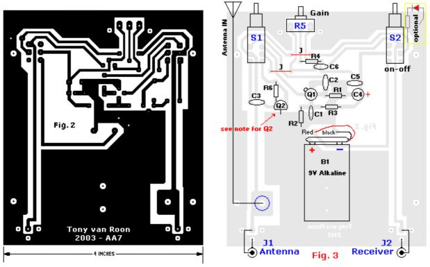
**Fig. 2.** "The AA-7 was assembled on a printed-circuit-board (PCB), measuring about 4 by 4-11/16 inches. A template for the printed-circuit-board is shown here. Note that it may not be to scale.
