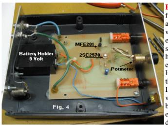
Fig. 4. shows the finished assembly without the enclosure. Make sure the antennahole in the enclosure is inline with one on the pcb. On mine I used a stud with thread on both sides to enable me to use
